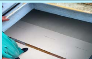
Ship-bottom wear plates
